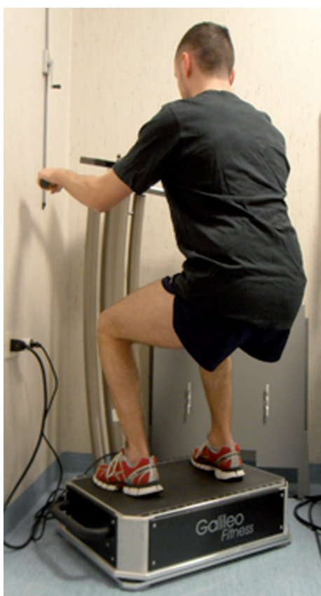
Figure 1.—The Galileo platform (Novotec Medical GmbH, Germany) used for WBV training oscillates around a central axis. A crankshaft principle on each side of the platform translates the rotating motion of the electromotor into a vertical displacement, inducing a seesaw vibration.
