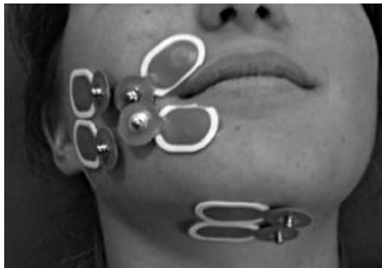
Figure 1.—Positioning of sEMG electrodes respectively for masseter, orbicularis oris and submental muscles
